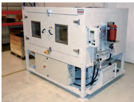
Pressure pulsation test rigs
