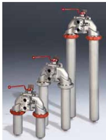
For continuous operation up to 100 bar operating pressure, the reversible variant is suitable, which consists of two filter housings with ball-valve switching. Otherwise this version corresponds to the PFL / PFM / PFH series. If desired, both side parts can be monitored by a central clogging indicator.
