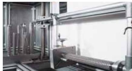
Final inspection on the bubble point test bench. Only filter candles in perfect condition leave our factory.
