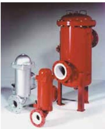
Comprehensive inline filter series for flow rates up to 25,000 l/min. Housing material: spheroidal graphite cast iron EN JS 1030 or carbon steel or made entirely of stainless steel. Flange connections from DN 50. Depending on the size, the pressure stage is PN 25 or PN 16 bar. The element technology corresponds to the series PRFLD.
