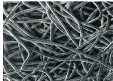
Chemicon® is a renewable metal fibre depth filter medium whose three-dimensional structure gives it a high contaminant-absorption capacity and excellent retention properties. Optimal media resistance and temperature resistance up to 400 °C thanks to austenitic material 1.4404.
