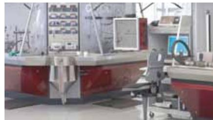
Standardised test procedures for our filter elements ensure consistently high filter performance. The filtration performance and contamination retention capacity are tested on our multi-pass test bench.
