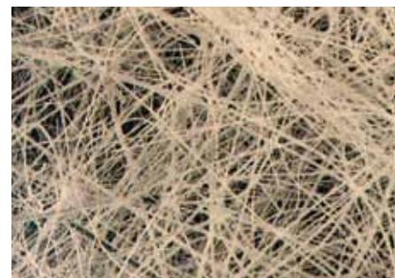
This disposable filter material is characterised by a very high contamination retention capacity with low purchase costs.
