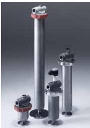
Universal filter made of stainless steel for pressures up to 100 bar, temperatures up to 200 °C and flow rates up to 120 l/min. Connection size: Cylindrical pipe thread G 1". Great variety of applications thanks to numerous sizes. Filter materials: slotted tube, wire mesh, Chemicon® metal fibre, coiled plastic candles. Special feature: no tools are required for element dismantling.
