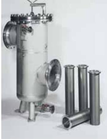
Screen basket filters are used mainly as coarse filters or pre-filters. Unlike the inline filters PRFL and PRFLD, the direction of flow is from the inside to the outside. The separated solids remain behind in the stainless steel strainer and can be removed easily and quickly. Nominal widths of DN 50 and larger are available. Materials: carbon steel or stainless steel 1.4571.
