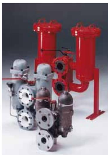
To avoid operation interruptions when elements are changed, change-over filters are suitable, in which one housing is in filtration and the other is in reserve. Switching is done by means of ball valves or flap switchover with a hand wheel. The special structure of the switchover organs prevents both filter housings from being blocked at the same time. The filter housings can be equipped with slotted tubes or filter candles made of wire mesh or glass fiber Betamicron®.
